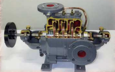
水道用送水ポンプ (断面模型) Circulating pump for tap water (X-section model)
